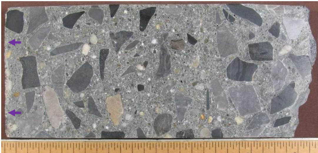
Figure 5 - This photograph is a lapped cross-section from Core 9 and illustrates the general appearance, distribution, and condition of the aggregates in the concrete. The top surface is oriented to the left. The 1-mm thick finished surface is indicated by purple arrows. The scale is in inches.
