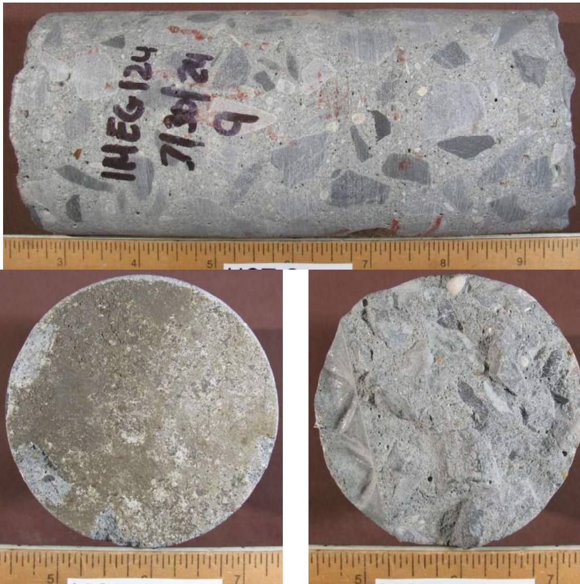
Figure 4 – Top: Core 9 as received for examination (top surface oriented to the left). Bottom: Top (left) surface indicating possible coring damage with blue arrows and bottom (right) surfaces of Core 9. Scales are in inches.
