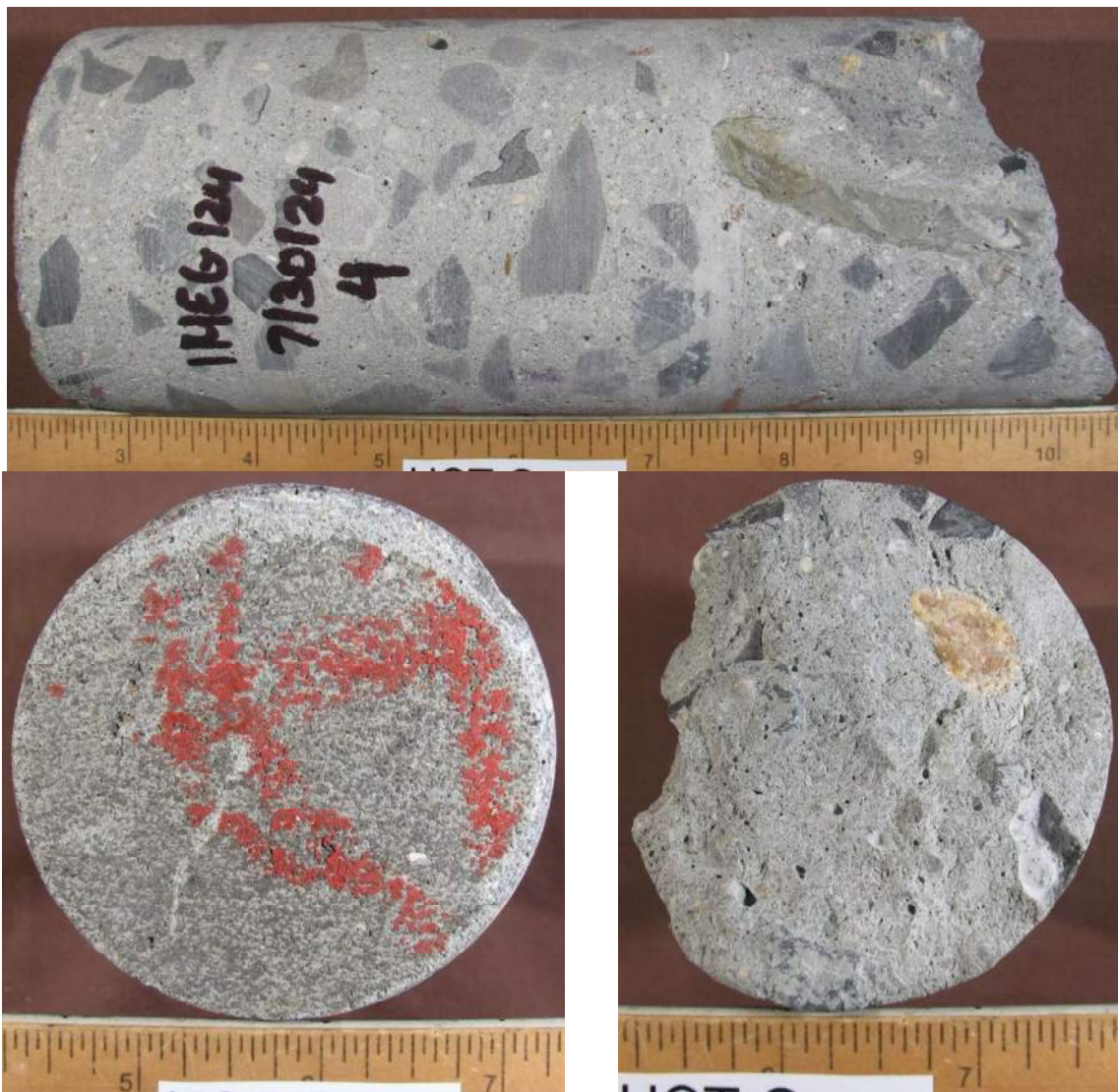
Figure 1 – Top: Core 4 as received for examination (top surface oriented to the left). Bottom: Top (left) surface with coring damage and bottom (right) surfaces of Core 4. Scales are in inches.
